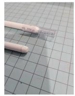
The Rod must be cut to length and then both ends will need to be rounded to eliminate any
